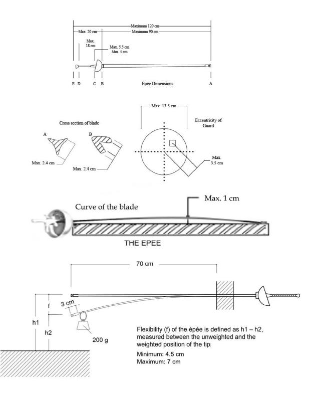
Figure 9. Epée dimensions and flexibility
