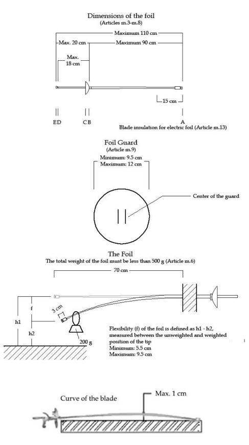
Figure 8. Foil dimensions and flexibility
