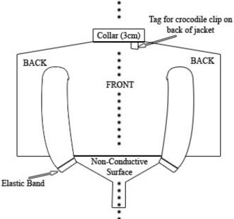
Figure 15. Electric sabre conductive jacket
