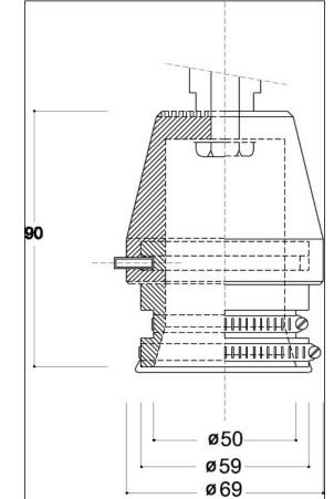
Figure A.5. Fixing device for test of cloth resistance to perforation
